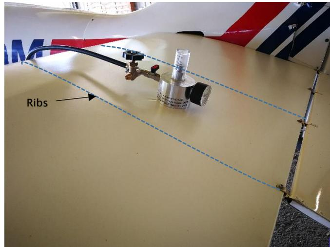
*Figure 4 Positioning of test head*
